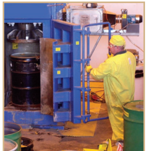
Volume reduction of compactible waste with Chase High Force Supercompactor.
